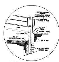
SUGGESTED ELEVATED RAMP EXIT INSTALLATION RAMP ELEVATION TO BE 16" ABOVE FINISH GRADE.
