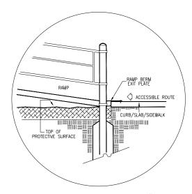
SUGGESTED RAMP BERM EXIT PLATE "8-16 INCH DECK TO GRADE/DB" INSTALLATION. REFER TO RAMP BERM EXIT PLATE INSTALLATION SHEET
